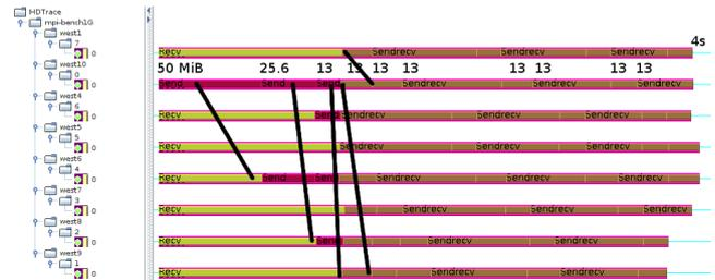
**Fig. 4** `MPI_Bcast()` of 100 MiB of data to 8 processes.
